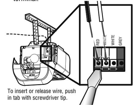
**PRE-WIRED INSTALLATIONS:** Connect the same wires to the garage door opener that were previously connected to the door control.
