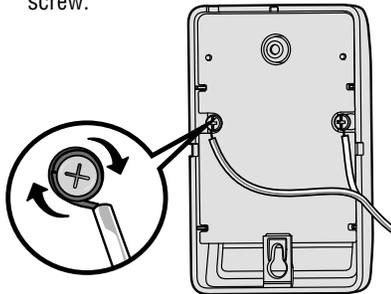
**PRE-WIRED INSTALLATIONS:** Choose any two wires to connect, but make note of which wires are used.
