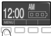
**2** Use the navigation buttons to scroll to "PROGRAM" and press the navigation button under **▶** to continue.
